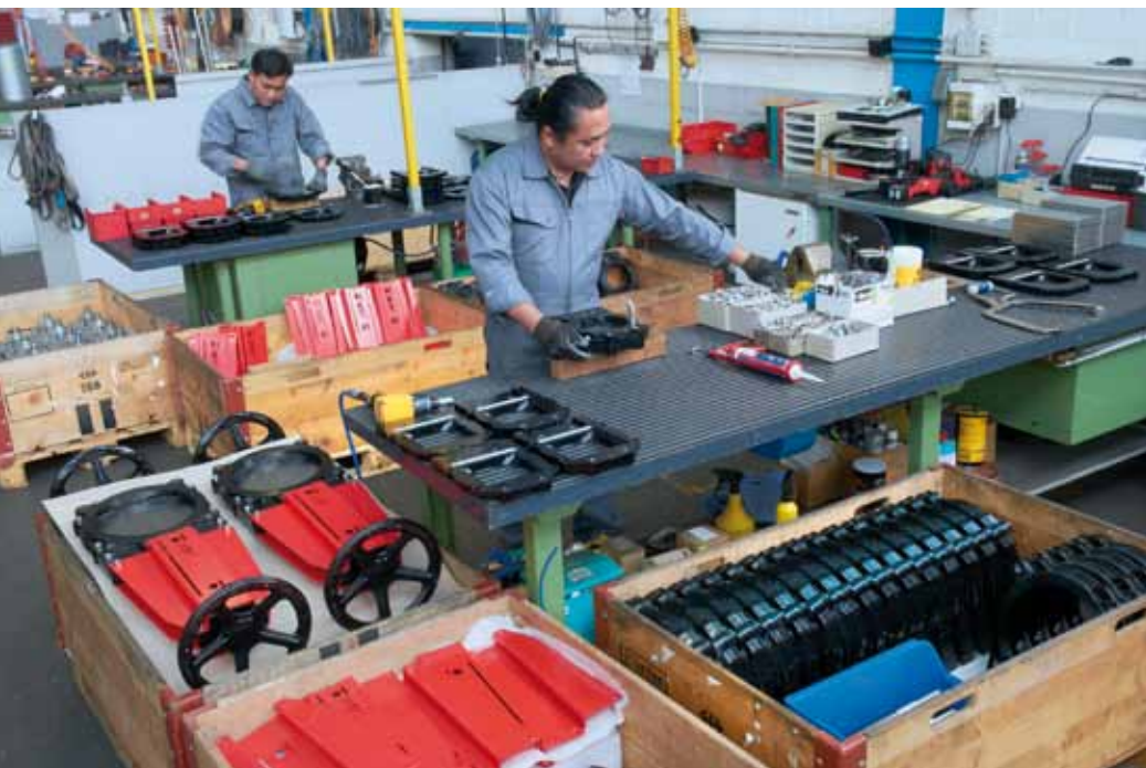
Assembling Wey Knife Gate Valves
